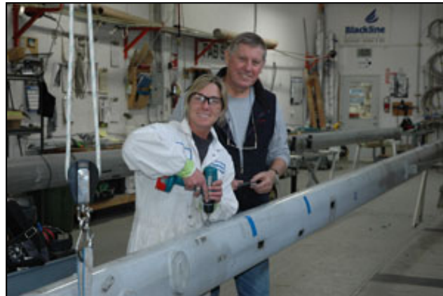
Second-year apprentice Candace Walmsley installs a new sail track on a refurbished mast section with the help of Campbell Black, owner of Blackline Marine. Photo by Blackline Marine
